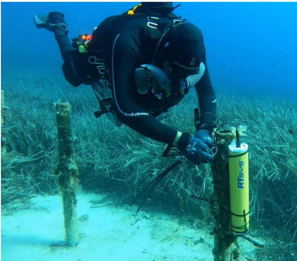
A CCR scientific diver deploying an underwater sound recorder in shallow water. Photo VLIZ – Sven Van Haelst
